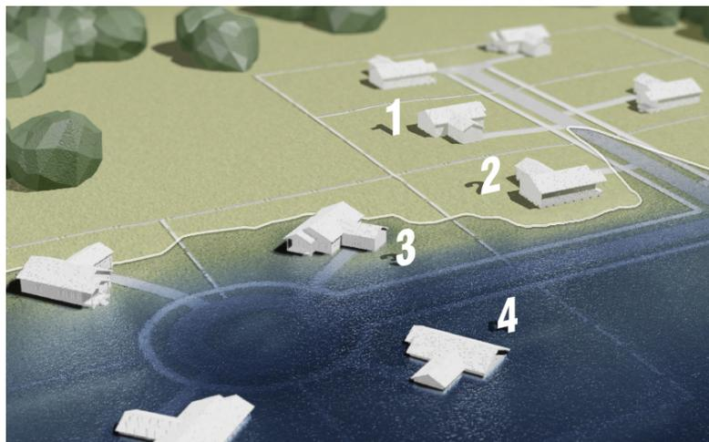
Base Flood illustration - where water surface elevation = BFE.
